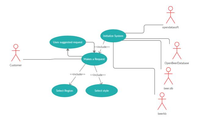
This diagram represents our secondary basic flow. In this diagram, after the system has initialized, a user will make their request, eliminating the beer by style and region. After this the system will return a list and prompt the user to see if they want to make a new request based off of a suggested request. This will then do another query, and add this to the user's current list. This will continue until the user feels satisfied with their choices and leaves the system.
